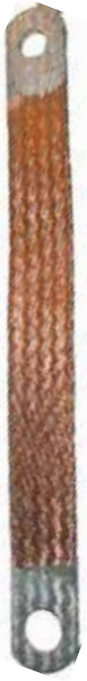
Use a ground strap instead of solid round wire for grounding. That addresses the skin effect so prominent in high-frequency VFD signals.
