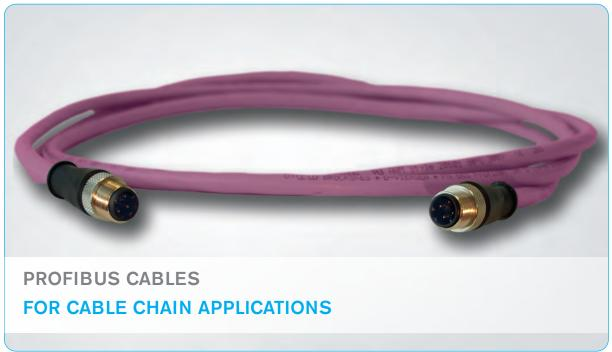
This assembly can be used for the field bus wiring in automation. These bus cables transfer Profibus signals with different cable and plug combinations. The PUR cable for cable track applications is resistant against rough environmental conditions in industrial applications.
