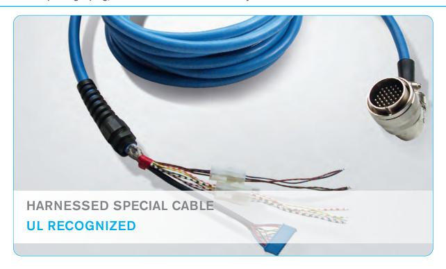
The example above is used in robotic applications, particularly for paint robots. This example has a 37-pole angle plug on the one side and an AMP Molex connector on the other side. The cable assembly can be adapted to the customer's requirements.
