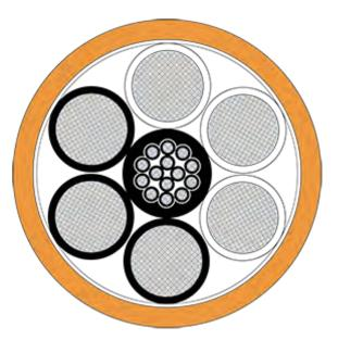
Application: For the application as fixed supply cable with optimised installation or for a flexible hand-held application without elevated mechanical stress for example mobile GPUs. Excellent flexibility due to smooth core and sheath materials make possible an easy laying and handling.
