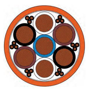
Application: For use as fixed cable with particularly good laying ability or for flexible use without high mechanical stress, e.g. in slow moving drag chains on passenger boarding bridges. Optimized flexibility due to flexible core and jacket materials, thus easy installation and easy handling in the cable dispenser. Depending on the operating conditions, it can also be used as a direct supply line to the aircraft with a connector.
