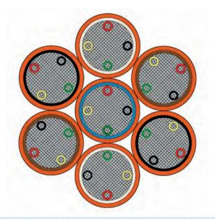
Application: Symmetrical cable with high flexibility. Minimum bending radius (easy to coil even in tight spaces) and high quality electrical performance (low voltage drop and low voltage unbalance). Can be used in long lengths.
