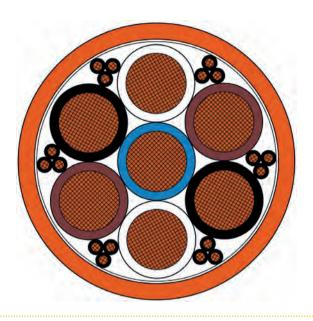
Application: For use as fixed cable with particularly good laying ability or for flexible use without high mechanical stress, e.g. in slow moving drag chains on passenger boarding bridges. Optimized flexibility due to flexible core and jacket materials, thus easy installation and easy handling in the cable dispenser. Depending on the operating conditions, it can also be used as a direct supply line to the aircraft with a connector.
