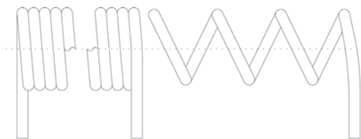
Helical direction ⇨ right (clockwise)
