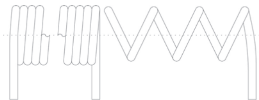
Helical direction ⇨ left (counter-clockwise)
