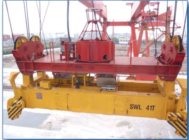
spreader power cables
